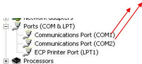
※ If your PC does not have Serial COM Port, install USB2Serial converter. USB2Serial converter is a device that converts USB port to Serial COM Port and can be easily found in PC accessory corners.
