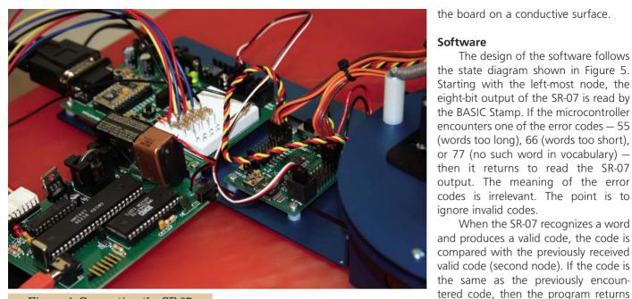
Figure 4. Connecting the SR-07 and the Board of Education on the robot arm.
